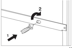
When placing the appliance ensure that it stands level. This can be achieved by two adjustable feet at the bottom in front.
